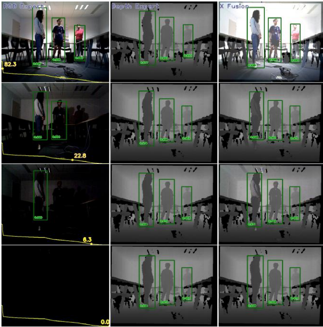
Fig. 7. Influence of decreasing luminosity. ONERA.ROOM propose a static sequence where the only changing factor is ambient light. The yellow curve indicate the mean pixel intensity. First column shows true positive detection of RGB expert, second column concerns depth expert and third column are the X-fusion detections. The last column images are made from the RGB and depth mean image for illustration purpose only.
